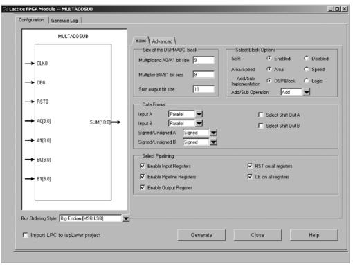
Figure 13-7. MULTADDSUB Mode Advanced Set-up
