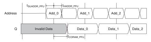
Figure 10-47. PFU Based ROM Timing Waveform – with Output Registers
