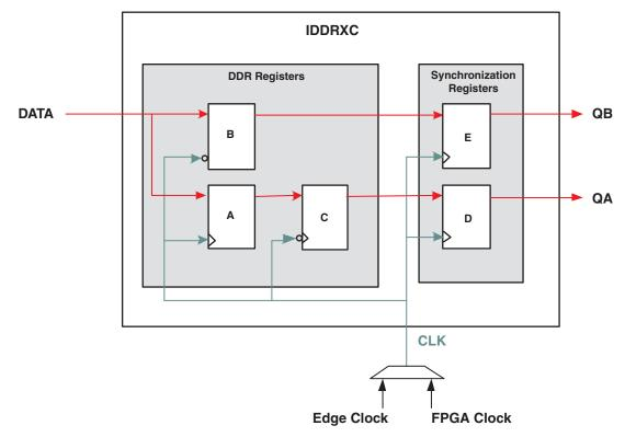
Figure 11-27. Input Register Block Configured as IDDRXC
