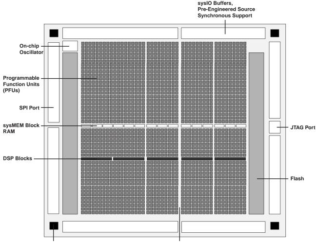
Figure 10-1. Simplified Block Diagram, LatticeXP2 Device (Top Level)
