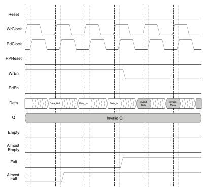
Figure 10-35. FIFO\_DC with Output Registers, End of Data Write Cycle
