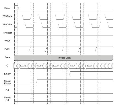
Figure 10-33 show the behavior of non-pipelined FIFO\_DC or FIFO\_DC without output registers. When we pipeline the registers, the output data is delayed by one clock cycle. There is an extra option for the output registers to be enabled by the RdEn signal.
