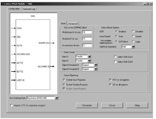
Figure 13-5. MAC Mode Advanced Set-up
