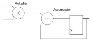
This block diagram can be mapped directly into the sysDSP primitives. Note that if a test point were added between the multiplier and the accumulator, or two output registers, etc. the code could not be mapped into a MULT18X18MACB of a sysDSP Block. Therefore, options that could be included in a design are input registers, pipeline registers, etc. For more Inferring design examples refer to EXAMPLES in the ispLEVER software.
