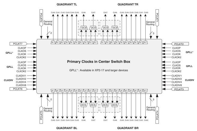
Figure 9-23. LatticeXP2 Primary Clock Muxes
