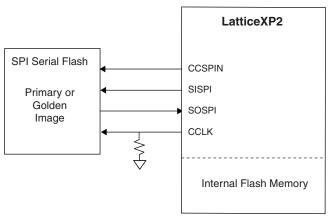
Internal logic is used to detect a configuration failure from the primary source and provides the ability to reattempt configuration from the secondary source. This sequence is used when the LatticeXP2 is set to dual boot mode and configuration is initiated.
