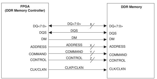
Figure 11-2. Typical DDR2 SDRAM Interface
