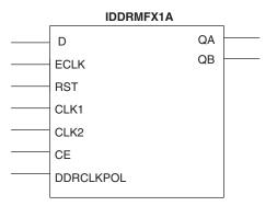
Table 11-4 provides a description of all I/O ports associated with the IDDRMFX1A primitive.
