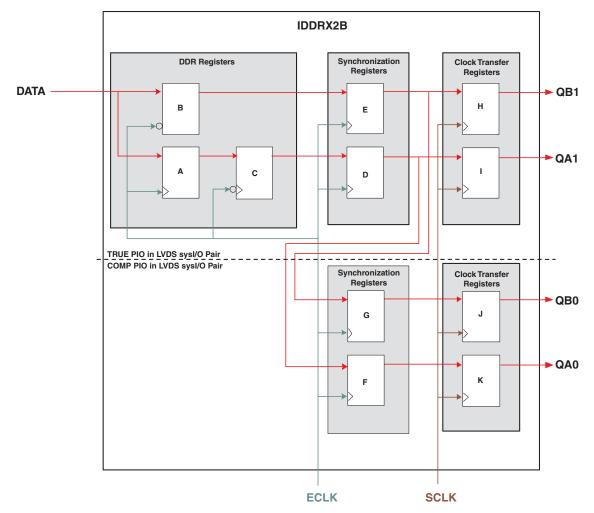
Figure 11-33. Input Register Block Configured as IDDRX2B
