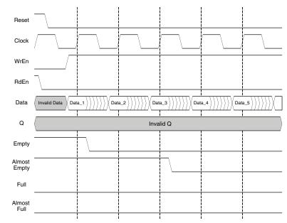
Figure 10-25. FIFO with Output Registers, Start of Data Write Cycle
