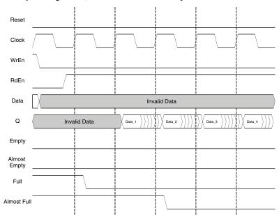
Figure 10-27. FIFO with Output Registers, Start of Data Read Cycle
