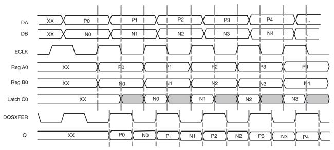
Note that the DQSXFER is inverted inside the ODDRXMA. This will cause the data coming out of the ODDRXMA to be -90° in phase with the output of the ODDRXC module.
