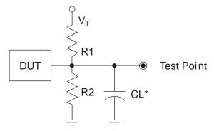
\*CL Includes Test Fixture and Probe Capacitance
