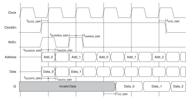
Figure 10-6. Single Port RAM Timing Waveform - NORMAL Mode, without Output Registers
