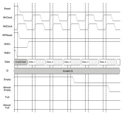
The WrEn signal must be high to start writing into the FIFO\_DC. The Empty and Almost Empty flags are high to begin and Full and Almost full are low.
