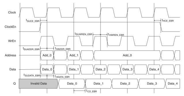
Figure 10-8. Single Port RAM Timing Waveform - WRITE THROUGH Mode, without Output Registers
