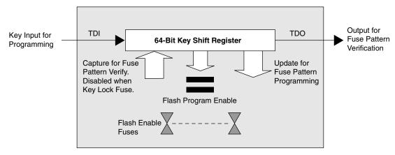
The next highest level of security for the LatticeXP2 is the 64-bit Flash Protect feature. The 64-bit Flash protect key is used to protect the embedded configuration flash from accidental or unauthorized erasure or reprogramming. This feature does not prevent the device from read back. Therefore, user is given the option to turn ON the CONFIG\_SECURE feature.
