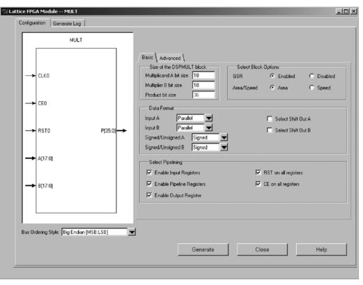
Figure 13-3. MULT Mode Advanced Set-up
