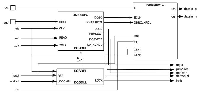
Figure 11-20. Software Primitive Implementation for Memory READ (Full Clock Transfer)
