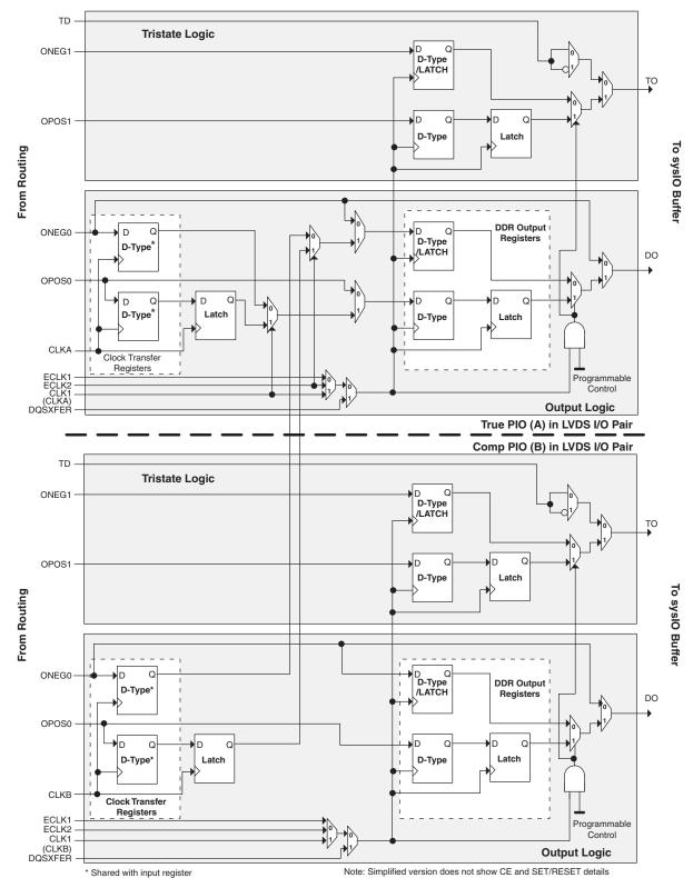
Figure 2-27. Output and Tristate Block
