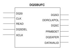
The DQSBUFC is composed of the DQS Delay, the DQS Transition Detect and the DQSXFER block as shown in Figure 11-8. This block inputs the DQS and delays it by 90 degrees. It also generates the DDR Clock Polarity and the DQSXFER signal. The preamble detect (PRMBDET) signal is generated from the DQSI input using a voltage divider circuit.
