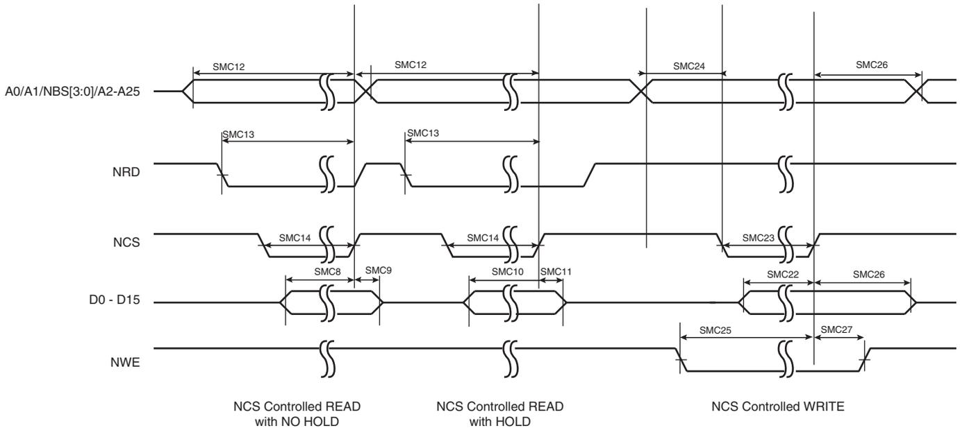
**Figure 43-26. SMC Timings - NRD Controlled Read and NWE Controlled Write**
