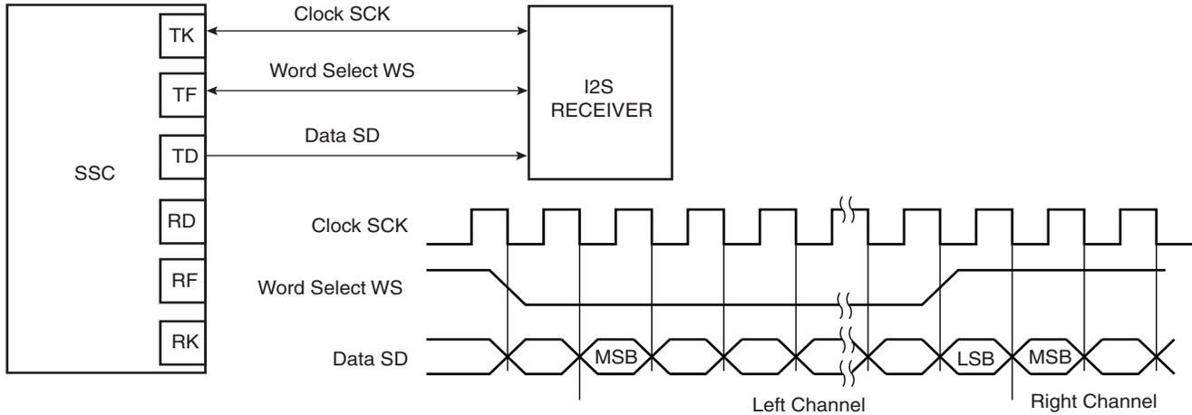
**Figure 31-18.** Codec Application Block Diagram
