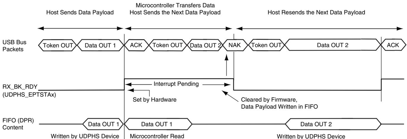
**Figure 39-14. Data OUT Transfer for an Endpoint with Two Banks**
