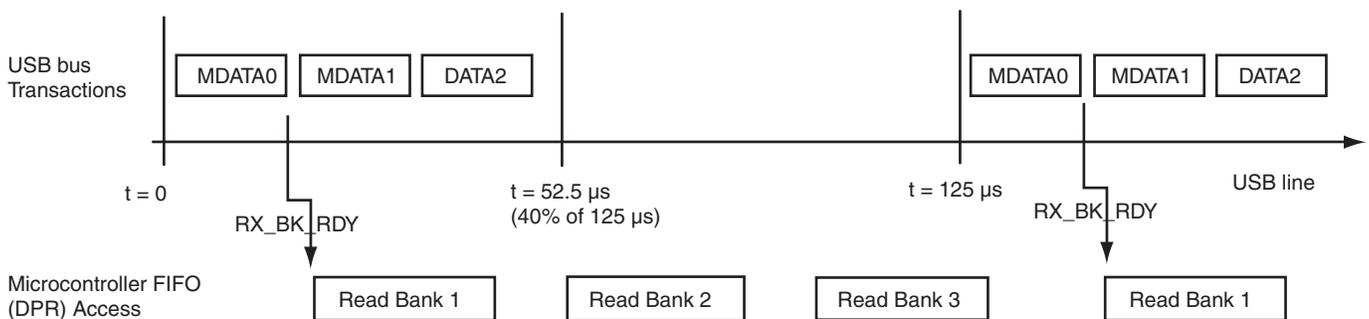
USB 2.0 supports individual High Speed isochronous endpoints that require data rates up to 192 Mb/s (24 MB/s):  $3 \times 1024$  data bytes per microframe.
