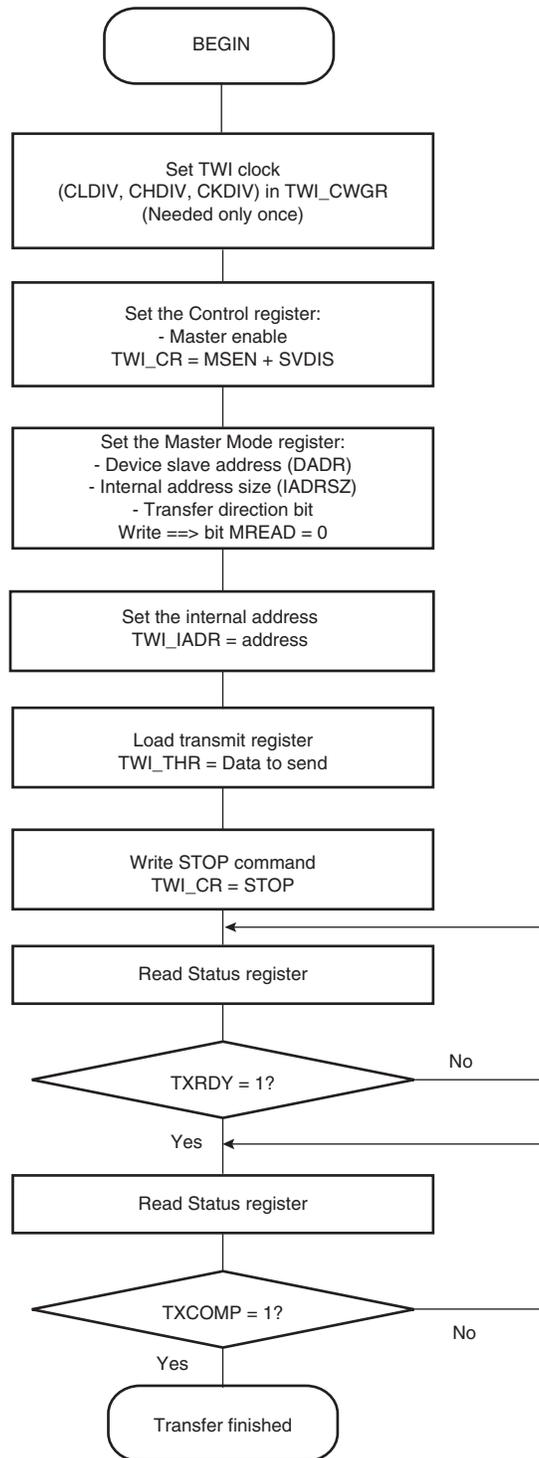
**Figure 33-18. TWI Read Operation with Single Data Byte without Internal Address**
