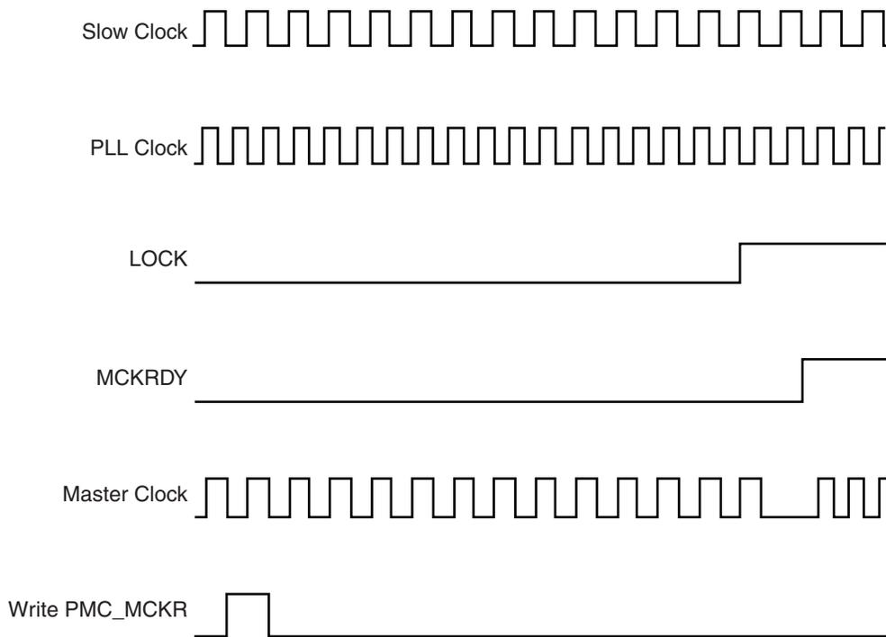
**Figure 28-5.** Switch Master Clock from Main Clock to Slow Clock
