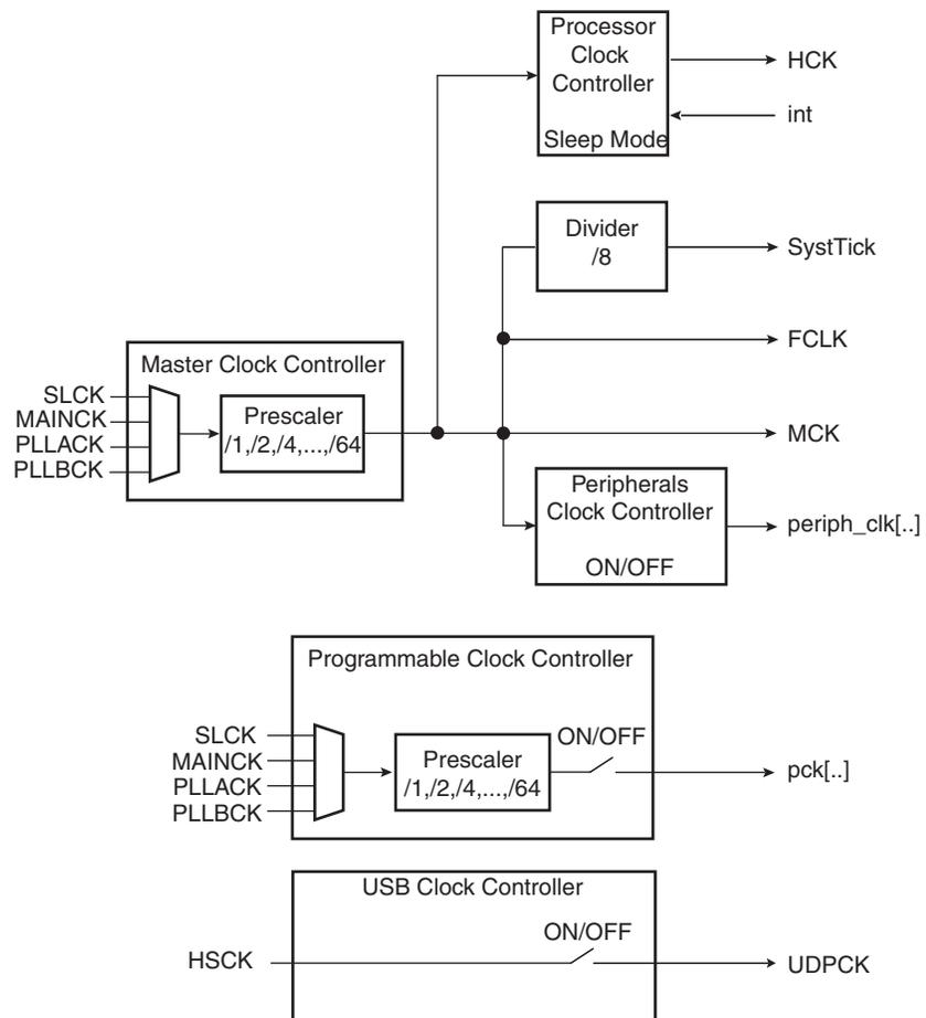
The SysTick calibration value is fixed at 10500, which allows the generation of a time base of 1 ms with SysTick clock to 10.5 MHz (max HCLK/8).
