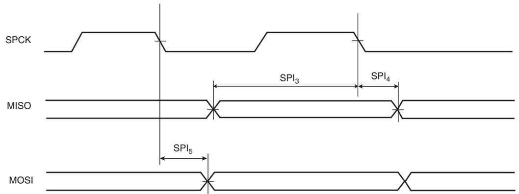
**Figure 43-14.** SPI Slave Mode with (CPOL=0 and NCPHA=1) or (CPOL=1 and NCPHA=0)
