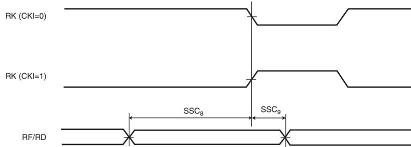
**Figure 43-21. SSC Receiver, RK as input and RF as output**
