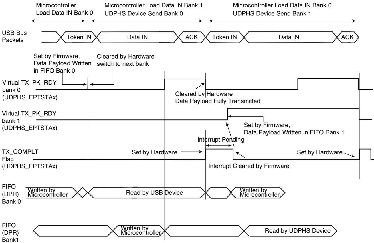
**Figure 39-10. Data IN Followed By Status OUT Transfer at the End of a Control Transfer**
