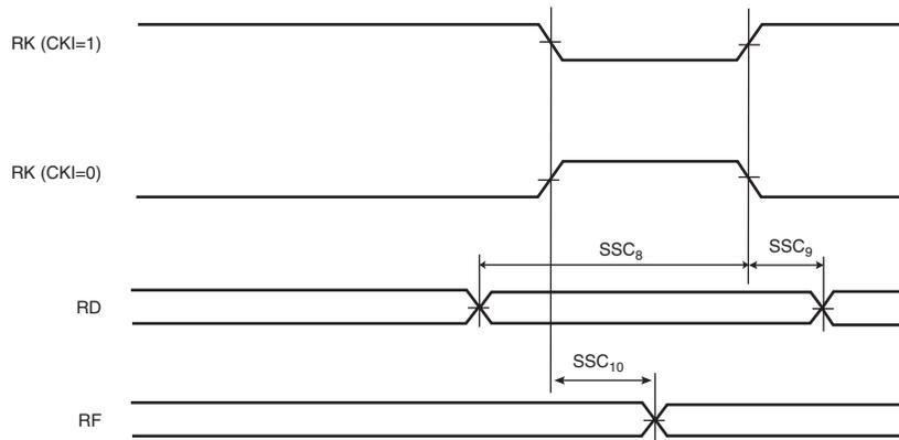
**Figure 43-22.** SSC Receiver, RK and RF as output
