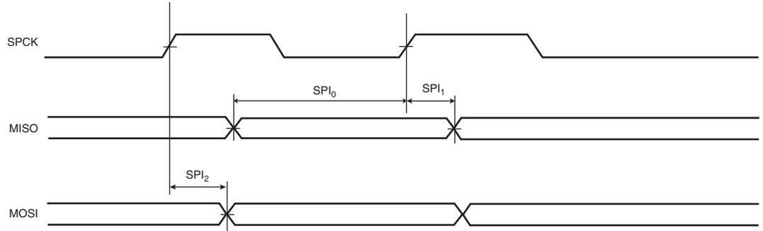
**Figure 43-13.** SPI Master Mode with (CPOL = 0 and NCPHA=1) or (CPOL=1 and NCPHA= 0)
