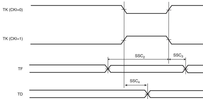
**Figure 43-19. SSC Transmitter, TK and TF as input**
