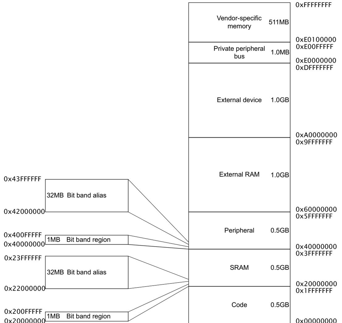
The regions for SRAM and peripherals include bit-banding regions. Bit-banding provides atomic operations to bit data, see [“Bit-banding” on page 72](#).
