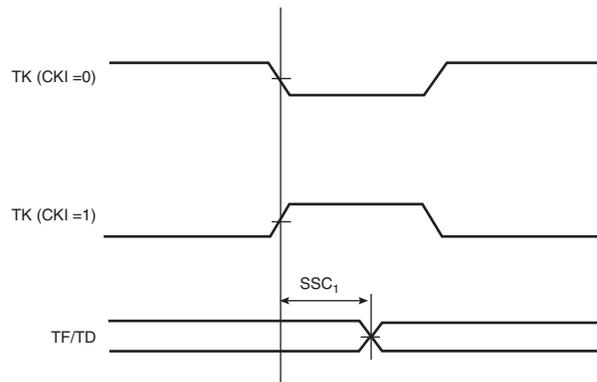
**Figure 43-18.** SSC Transmitter, TK as output and TF as input
