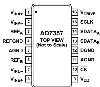
Figure 2. Pin Configuration
