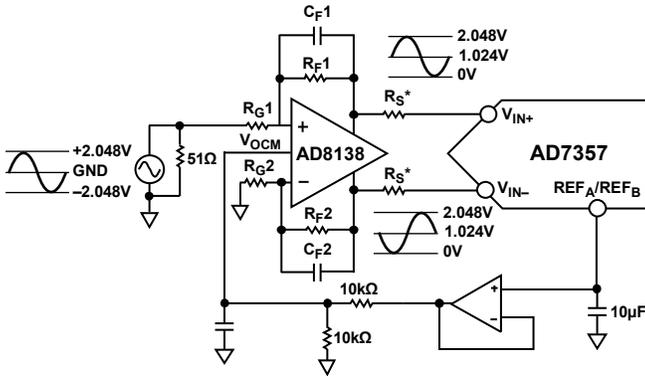
\*MOUNT AS CLOSE TO THE AD7357 AS POSSIBLE AND ENSURE THAT HIGH PRECISION  $R_S$  RESISTORS ARE USED.  $R_S = 33\ \Omega$ ;  $R_{G1} = R_{F1} = R_{F2} = 499\ \Omega$ ;  $C_{F1} = C_{F2} = 39\text{pF}$ ;  $R_{G2} = 523\ \Omega$
