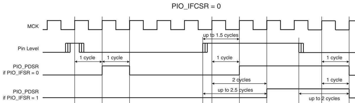
**Figure 30-6.** Input Debouncing Filter Timing
