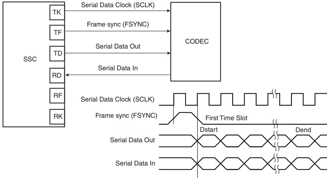
Figure 31-19. Time Slot Application Block Diagram
