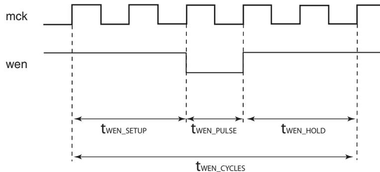
Figure 25-33. Write Enable Timing for NAND Flash Device Data Input Mode.
