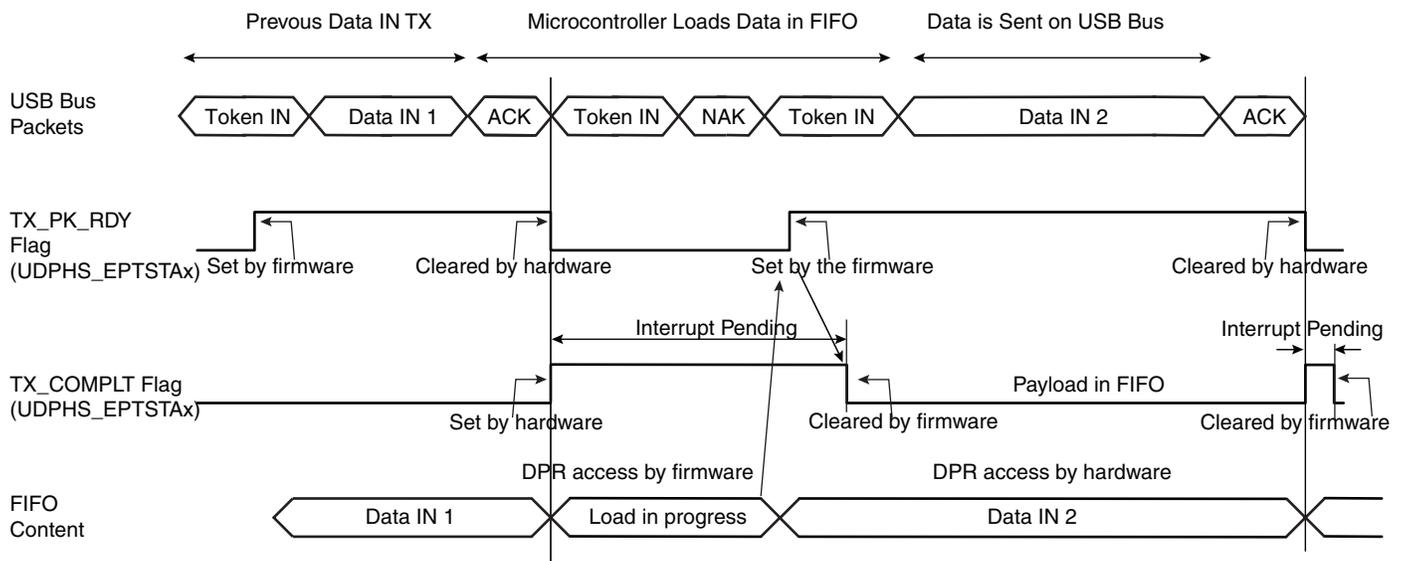
**Figure 39-9. Data IN Transfer for Endpoint with Two Banks**
