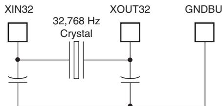
The user can set the Slow Clock Crystal Oscillator in bypass mode instead of connecting a crystal. In this case, the user has to provide the external clock signal on XIN32. The input characteristics of the XIN pin under these conditions are given in the product electrical characteristics section.
