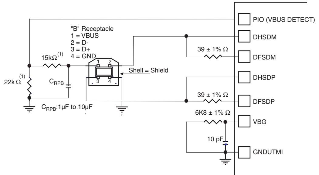
Note: The values shown on the 22 k $\Omega$  and 15 k $\Omega$  resistors are only valid with 3V3 supplied PIOs. Both 39  $\Omega$  resistors need to be placed as close to the device pins as possible.
