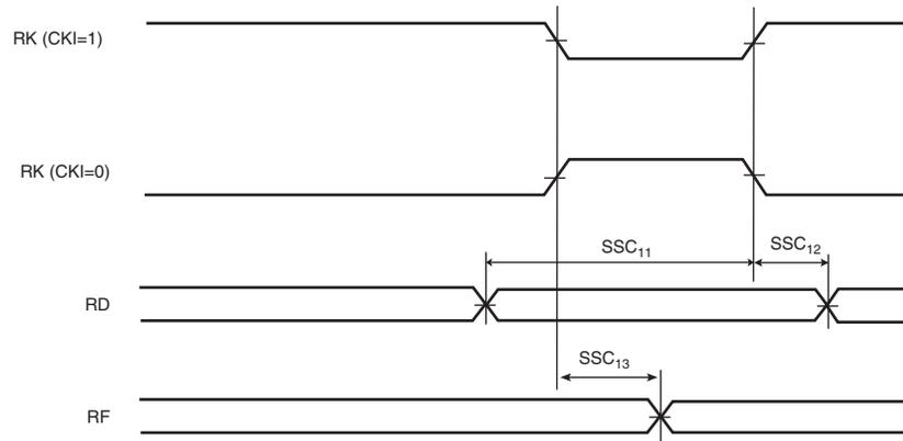
**Figure 43-23.** SSC Receiver, RK as output and RF as input
