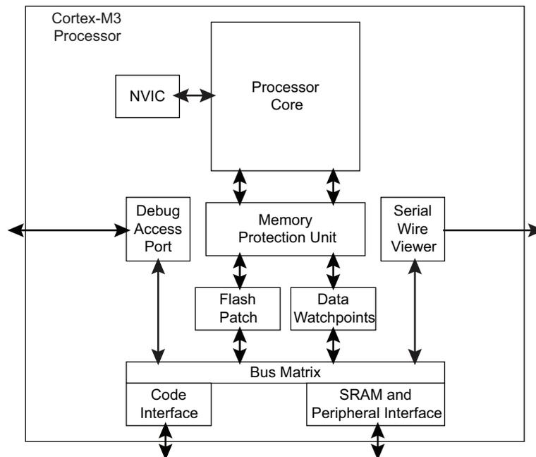
The Cortex-M3 processor is built on a high-performance processor core, with a 3-stage pipeline Harvard architecture, making it ideal for demanding embedded applications. The processor delivers exceptional power efficiency through an efficient instruction set and extensively opti-
