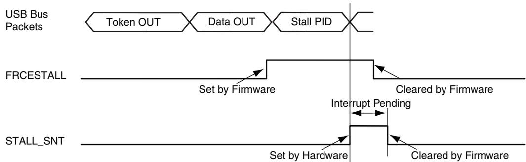
**Figure 39-17.** Stall Handshake Data IN Transfer
