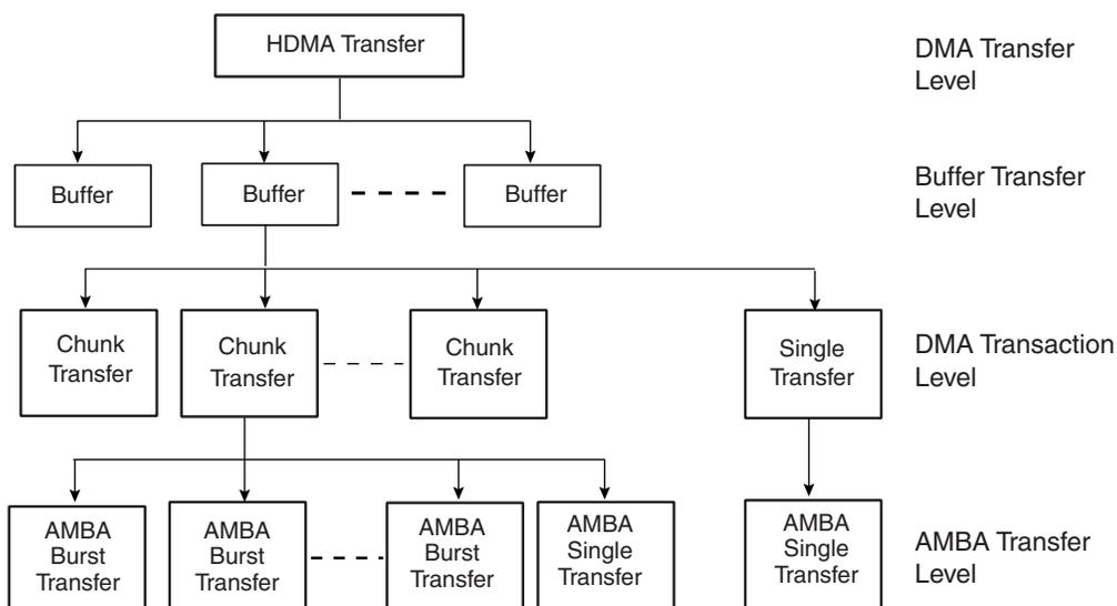
**Figure 40-3.** DMAC Transfer Hierarchy for Memory
