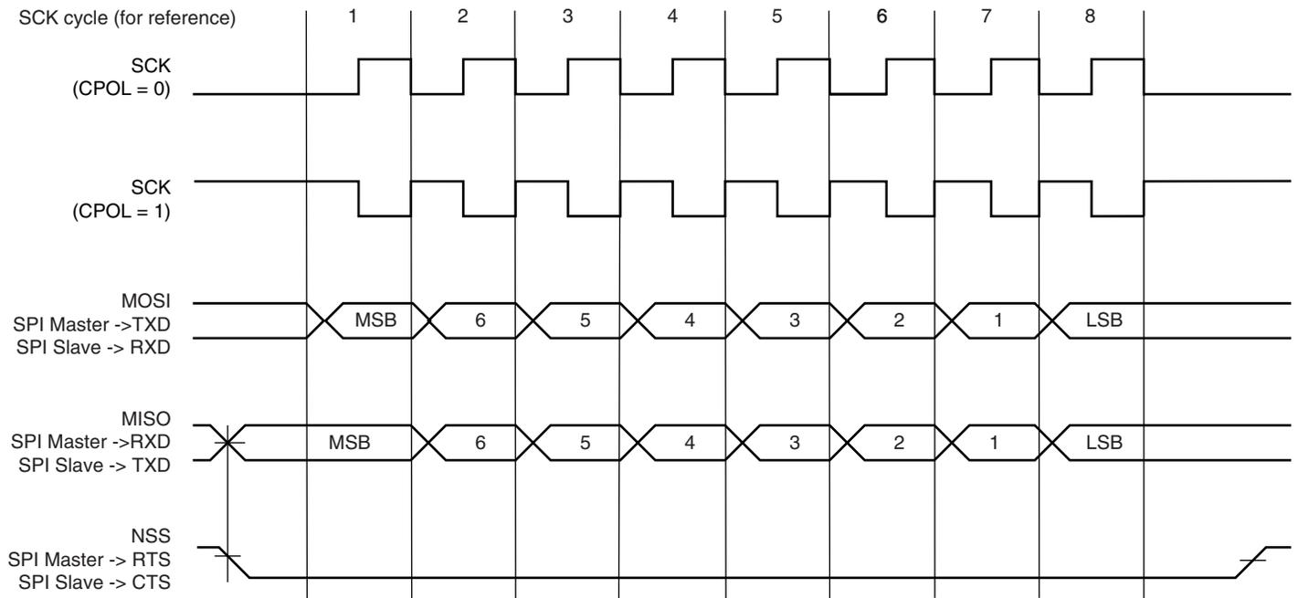
**Figure 35-39. SPI Transfer Format (CPHA=0, 8 bits per transfer)**
