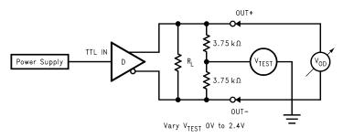
Figure 3. Differential Driver Full Load DC Test Circuit
