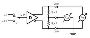
Figure 2. Differential Driver DC Test Circuit
