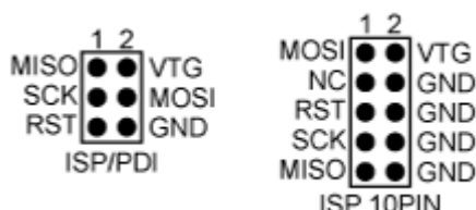
Figure 4-1. Connections for the 6- and 10-pin ISP Headers
